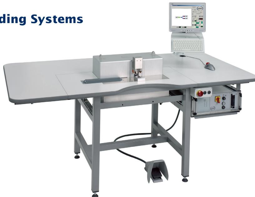
The ultrasonic welding system LS-60 is an economical and extremely robust production system for welding copper splices. Its 4kW-generator enables the processing of splices with cross-sections between 10 and 60 mm<sup>2</sup>. Under certain conditions, it is even possible to weld cross-sections that are larger than 60 mm<sup>2</sup>.
